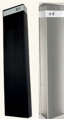
Samples after GM Alkaline resistance test pH 12.5
